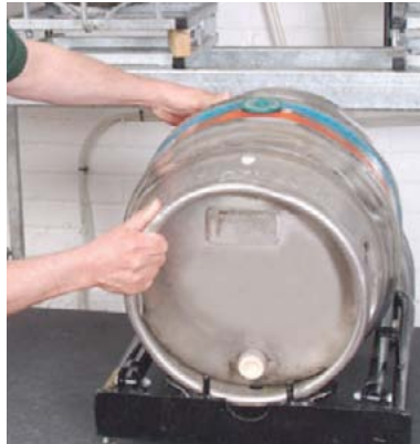
Stillaging: Leave for 24 hours after arrival to bring the barrel down to cellar temperature.
